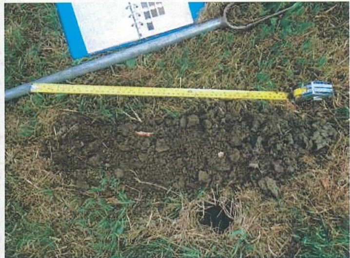
Left: soil materials in B horizon, TP#2 showing low chroma colors (2.5 3/1) at depths of less than 16 inches; Below: soil profile shot of TP#3 showing redox concentrations in upper part along with generally low chroma colors; note all materials silt loam
