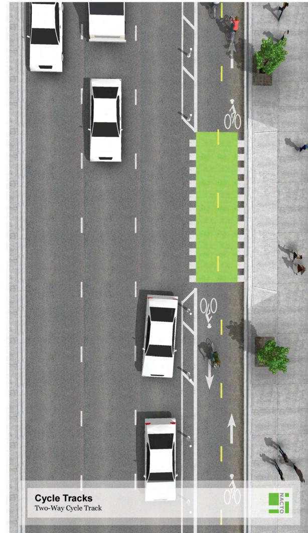
Figure 48: Protected Two Way Cycle Track Overhead, NACTO
