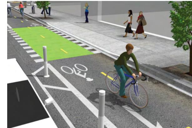
Figure 49: Protected Two Way Cycle Track, NACTO
