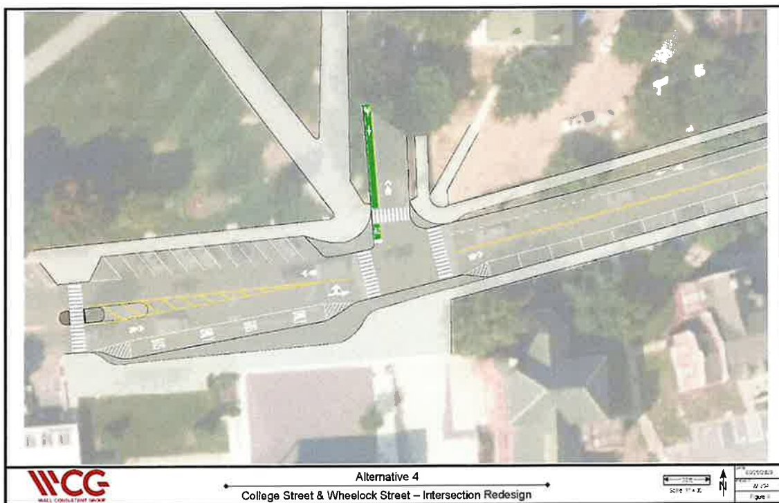
FIGURE 2: PREFERRED ALTERNATIVE (ALTERNATIVE 4 - REDESIGNED SMALLER INTERSECTION)
