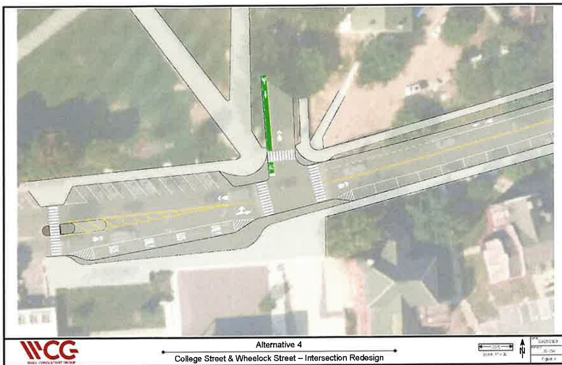
FIGURE 2: PREFERRED ALTERNATIVE (ALTERNATIVE 4 - REDESIGNED SMALLER INTERSECTION)
